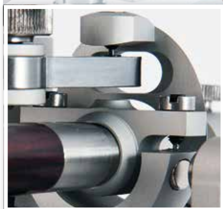
ABOVE/INSET: Horizontal movement is governed by a single unipivot [top of inset pic] while vertical movement is accommodated by two unipivots either side of the arm [under the screw heads]. Pivot stabilisation, and bias compensation, is achieved via chromed magnets that are inserted into the alloy yoke
