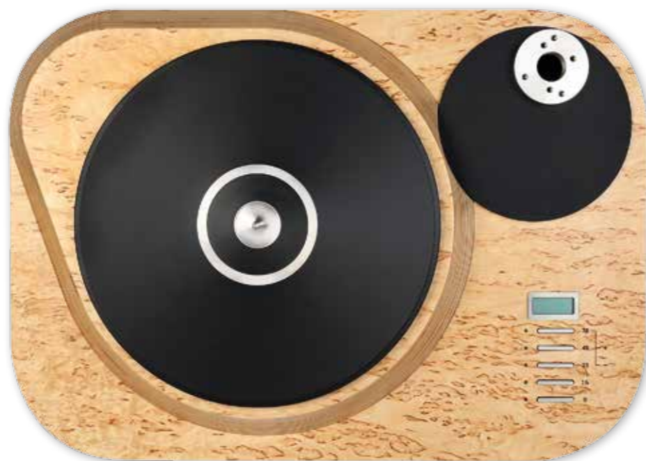
RIGHT: The slender platter and raised centre section allows the rim-drive mechanism [see boxout, p49] to be housed without resorting to inelegantly thick plinth. Arm mount hosts 9.5-12in types while speed control LCD also facilitates an electronic inclinometer
