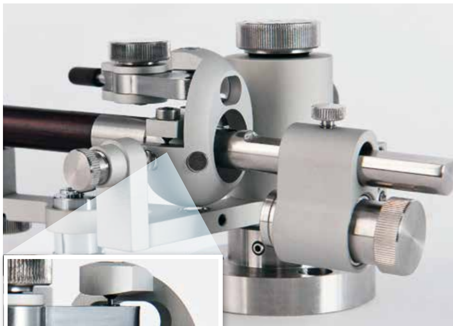
ABOVE/INSET: Horizontal movement is governed by a single unipivot [top of inset pic] while vertical movement is accommodated by two unipivots either side of the arm [under the screw heads]. Pivot stabilisation, and bias compensation, is achieved via chromed magnets that are inserted into the alloy yoke
