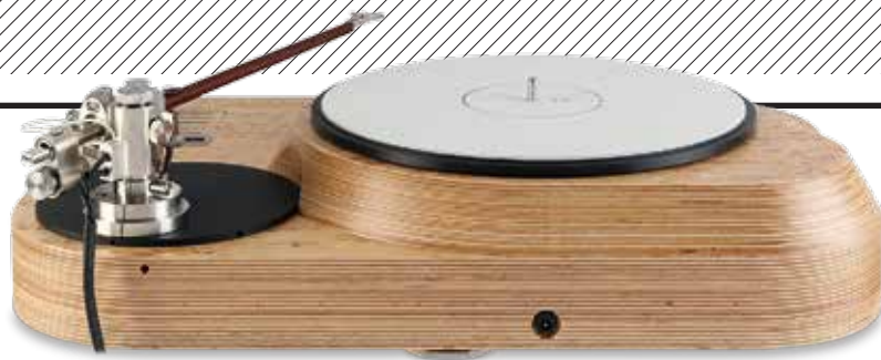
ABOVE: The 3P's underslung counterweight lowers the centre of gravity, further improving the stability of its 'multi-unipivot' bearing. The VTA/height adjustment dial is also easily accessible on the top pillar. The deck's 12V DC input socket is also visible
